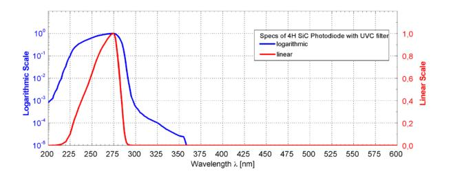
UVC-only SiC based UV photodiode A = 0.20 mm<sup>2</sup>
